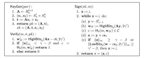
Fig. 3. Crystals-Dilithium signature scheme
