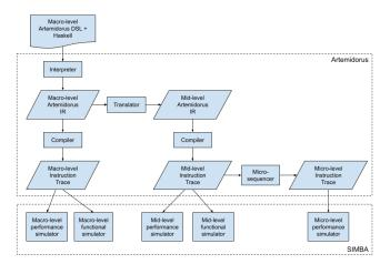
Figure 7: BASALISC Software Toolchain.
