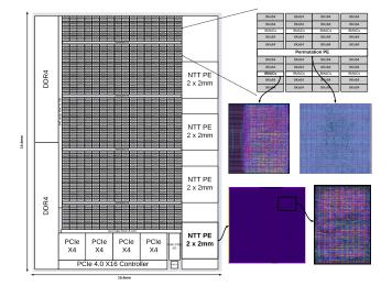
Figure 8: Floorplan of BASALISC 1.0 with all cells placed and intra-block routing complete. Note that the MAC PE and Permutation PE are interleaved within the CTB.
