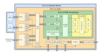
Figure 2: BASALISC 1.0 System Diagram.
