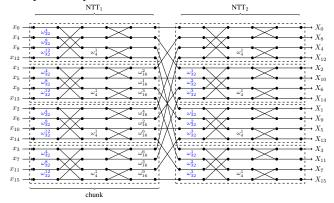
Figure 4: 16-point radix-4 negacyclic NTT flow graph. Extra negacyclic twiddles (in blue) are decomposed into two premultiply passes.
