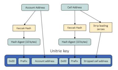
Figure 2: Unitrie key derivation from account and cell addresses.
