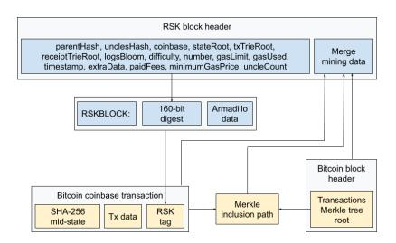
Figure 3: Placement of merged mining data in RSK and Bitcoin blocks.
