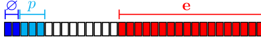
Figure 1: Plaintext binary representation with p = 8 = 2^3 (cyan), \pi = 2 (dark blue) such that 2^\pi \cdot p \leq q , the error e (red). The white part is empty. The MSB are on the left and the LSB on the right.
