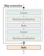
Fig. 2: Skip connection for residual network.
