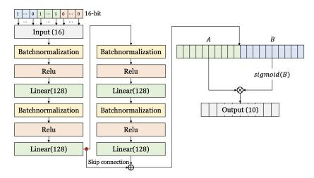
Fig. 6: Neural network structure for cryptanalysis for S-DES.
