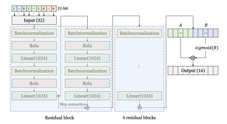
Fig. 7: Neural network structure for cryptanalysis for S-AES.
