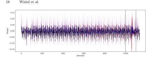
Fig. 4: 1,000 power traces of the FrodoKEM Gaussian sampler, modified to act as a two-sided sampler. Runs resulting in a negative sample are drawn in red, others in blue. The section marked by vertical lines shows the section used for training the classifier.
