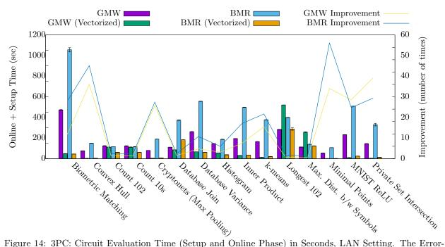
Figure 14: 3PC: Circuit Evaluation Time (Setup and Online Phase) in Seconds, LAN Setting. The Errorbars are Standard Deviation.
