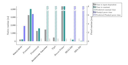
Fig. 1. Runtime comparison of different hash functions. The benchmarks are from Table 3 and the numbers for Monolith-64, POSEIDON, and POSEIDON2 are taken for the 64-bit prime field and a state size of t = 12 (sponge mode). Proof times are benchmarks for a proof of preimage knowledge (Table 5). Numbers for SHA3-256 and SHA-256 are extrapolated from a circom implementation using R1CS [Bal23].
