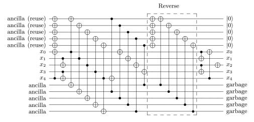
Fig. 2: ASCON S-box implementation in quantum (Toffoli depth 1).
