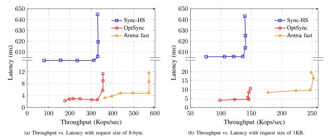
Figure 5: Throughput vs. Latency  $(n = 3, f = 1, \Delta = 300 \text{ms})$ .
