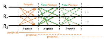
Figure 1: Communication patterns for pipelined Arena.
