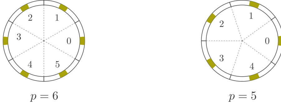
Fig. 5: Distribution of the values of \mu across \mathbb{Z}_q for p = 6 and p = 5 : the colored parts show the dense spots where the value has a high probability to lie in. The width of these sectors depends on \sigma (the standard deviation of the error distribution \chi of TFHE). Note that this repartition looks the same for \tilde{\mu} in \mathbb{Z}_{2N} .
