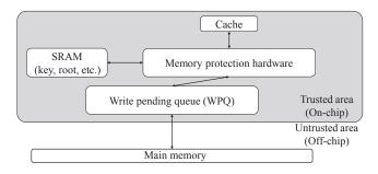
Figure 1: System model of encrypted memory, with focus on memory controller (CPU core(s) are omitted).
