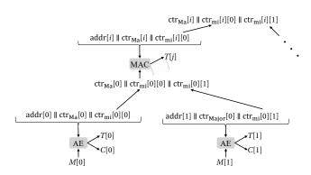
Figure 3: Example of SC-based binary PAT, where  $\operatorname{ctr}_{\mathsf{Ma}}[i]$  is i-th major counter, and  $\operatorname{ctr}_{\mathsf{mi}}[i][j]$  is j-th minor counter sharing  $\operatorname{ctr}_{\mathsf{Ma}}[i]$ . MAC input of parent node consists of major counter(s) and all minor counters of child nodes.
