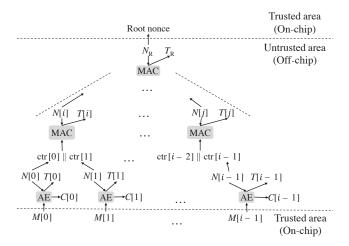
Figure 2: Overview of binary PAT. M[i], C[i], N[i], and T[i] denote plaintext (i.e., payload data), ciphertext, nonce, and tag of i-th node, respectively, where N[i] consists of address addr[i] and counter  $\operatorname{ctr}[i]$ .  $N_R$  and  $T_R$  are root nonce and tag, respectively. Leaf node is defined as (N[i], T[i], C[i]), whereas other nodes are defined as (N[i], T[i]).
