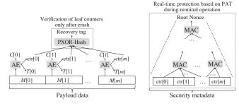
Figure 4: Secure memory based on PAT and Crystalor.
