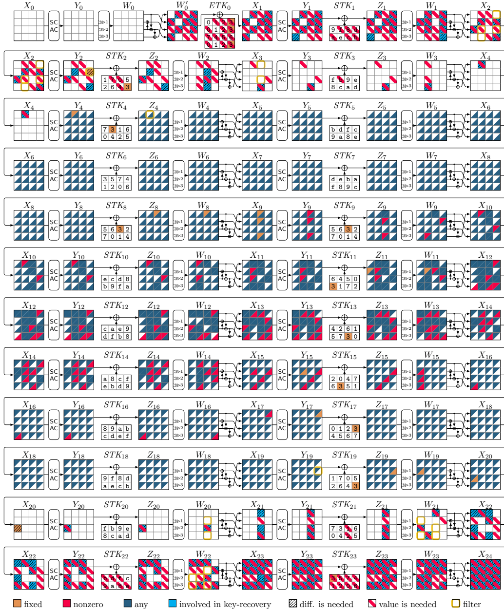
Figure 35: Related-Tweakey ID attack on 24 rounds of ForkSKINNY-128-256-256 in the limited setting ( r_i = 9, r_0 = 15 ). |k_B \cup k_F| = 224 , c_B = 56 , c_F = 96 , \Delta_B = 64 , \Delta_F = 96 . In this case we have 15 related-key impossible differences.
