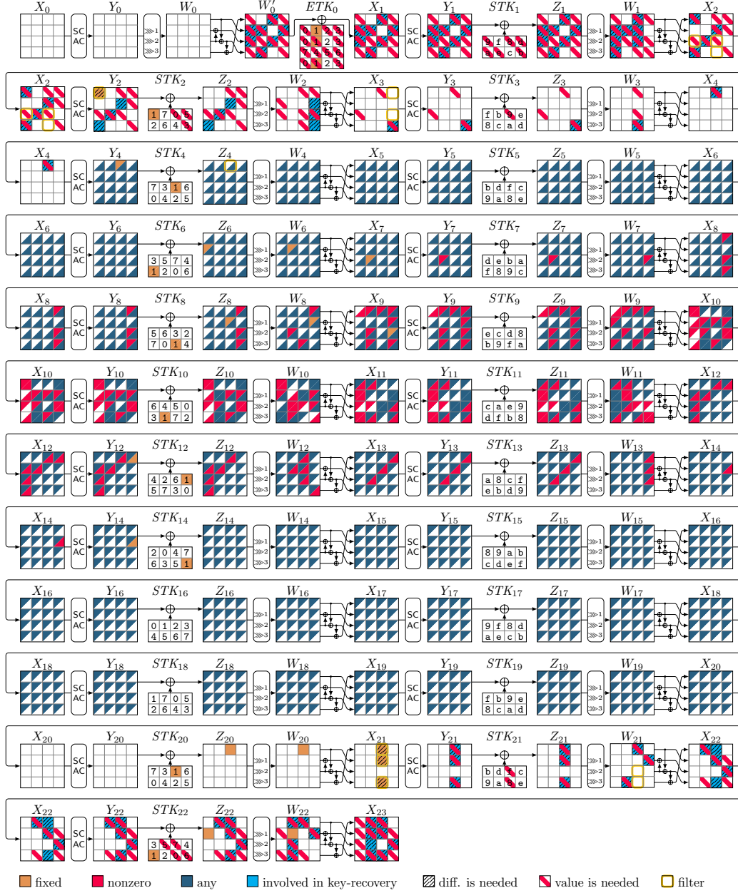
Figure 42: Related-Tweakey ID attack on 23 rounds of SKINNY128-288-128. |k_B \cup k_F| = 120 , c_B = 48 , c_F = 40 , \Delta_B = 56 , \Delta_F = 40 . In this case, we have 255 related-key impossible differences.
