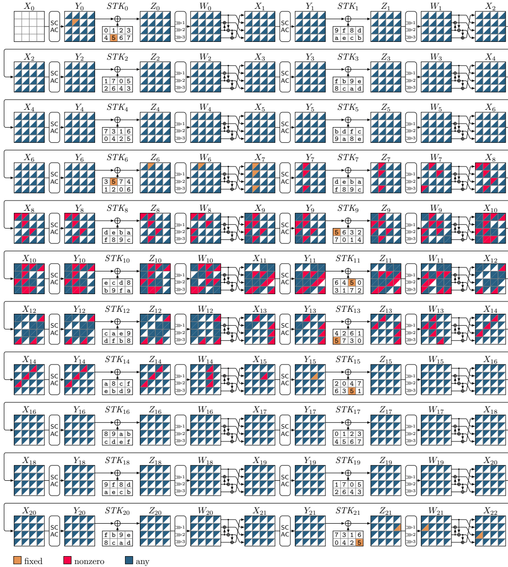
Figure 28: A cluster of 15 related-tweakey ID distinguishers for 22 rounds of ForkSKINNY-64-192, where r_i = 8 , r_0 = 15 , and r_1 = 14 .
