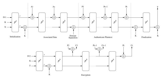
Figure 2: ASCON SIV encryption mode
