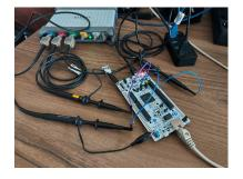
Figure 2: The Nucleo board and the PicoScope in the energy consumption configuration.
