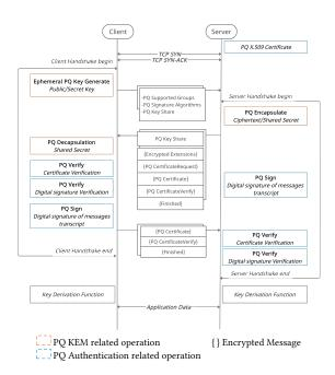
Figure 1: Post-quantum TLS 1.3 handshake messages.
