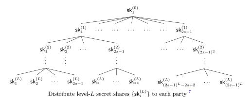
Fig. 3: High-level Overview of TreeSSS
