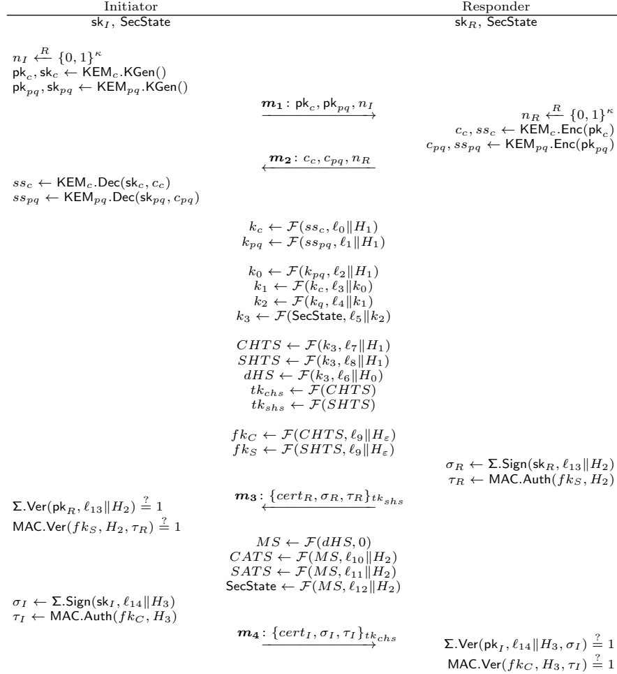
Fig. 2. One stage of the Muckle+ protocol. Messages \mathbf{m} : \{m_1, \dots\}_k denote that m_1, \dots is encrypted with an authenticated encryption scheme using the secret key k . The various contexts and labels are given in Tables 2 and 3.
