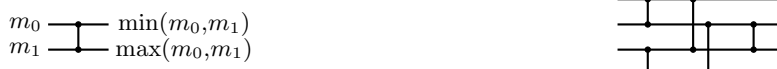
Fig. 1. The basic module and the network representation of odd-even merge sort for d = 4 .
