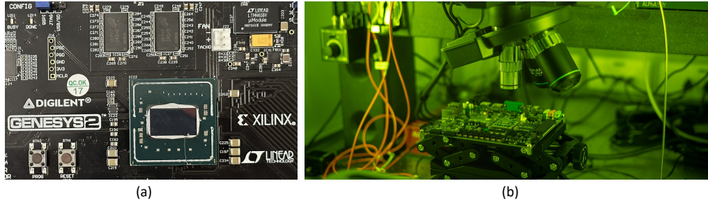
Figure 4: (a) The heatsink has been removed to get access the backside silicon of the FPGA. (b) The ALPhANOV InGaAs camera and microscope have been utilized for PEM.
