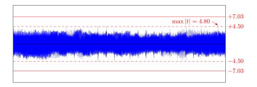
**Fig. 7.** 10,000 traces of the core signing process (SLH-DSA-SHAKE-128f) has a maximum spike at |t| = 4.80, which is below the critical value C = 7.03 with 4.91M time points. The secret keys are entirely handled by hardware, reducing their exposure to side-channel attacks.
