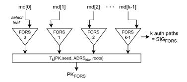
**Fig. 2.** Each SLH-DSA keypair defines  $2^h$  pseudorandom FORS keypairs; *idx* selects which one is used. FORS few-time signature generation uses *a*-bit segments of the message digest *md* to select leaf nodes in *k* Merkle trees. The trees have height *a* and are illustrated here with roots at the bottom. The authentication paths (hashes) to reach the roots from the leaves form the message signature SIG<sub>FORS</sub>.
