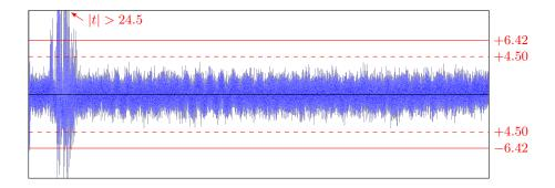
Fig. 5. A TVLA test of a processor implementation of SLH-DSA rapidly shows a leak of SK.seed secret key material. In this *t*-trace we captured the initial 73k cycles of the signing process, containing the first SHAKE256 **PRF** call. Maximum *t* value reaches 24.5 already in 1,000 traces. The SHA2-256 **PRF** exhibits similar leakage behavior.
