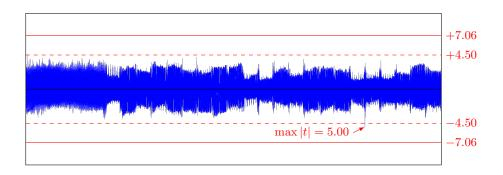
**Fig. 6.** 100,000 traces of the core signing process (5.95M cycles, one sample per cycle at 31.24MHz) has a maximum spike of |t| = 5.00, which is below the long-trace adjusted critical value C = 7.06.
