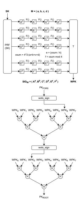
**Fig. 3.** Toy example of an XMSS hypertree signature, similar to the one in SLH-DSA. We illustrate WOTS (top) by signing an 8-bit message organized into four-bit pairs M = (a, b, c, d). Two additional checksum digits (e, f) are required. The hypertree (bottom) consists of d (here 2) layers of XMSS trees, each with a WOTS one-time signature authenticating the root of the previous layer.
