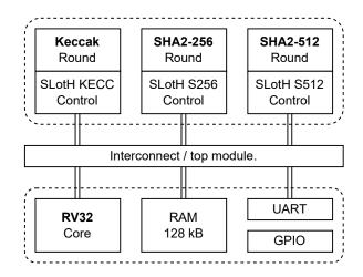
**Fig. 4. SLotH** consists of independent memory-mapped accelerators (top) and firmware that runs on a generic embedded RISC-V controller (bottom). In reality, the masked Keccak unit is currently a separate unit from the "normal" Keccak unit, but with equivalent functionality. The FPGA instantiations have simple UART and GPIO external interfaces, and 128kB of Block RAM to hold the firmware and work memory (stack). On RoT silicon, many parts of the firmware would be in mask ROM.
